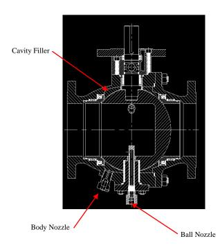
The body nozzle is available to flush sand and other media from the body cavity. The TFE cavity filler fills up most of the void in the body cavity so there is very little area to flush out. It is recommended that this port be used to flush the body once per month. To flush, first remove the set screw that is located in the Body nozzle with an allen wrench. Water or air can than be connected to perform the flush.
